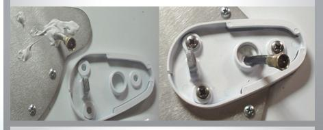
Apply sealant to 3 screws, fill coax hole, connect
